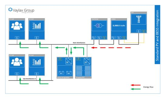
A standard grid-tied BESS attached to a consumer's infrastructure and accompanied by a PV system is technically designed to follow predefined or individual managed scenarios.
