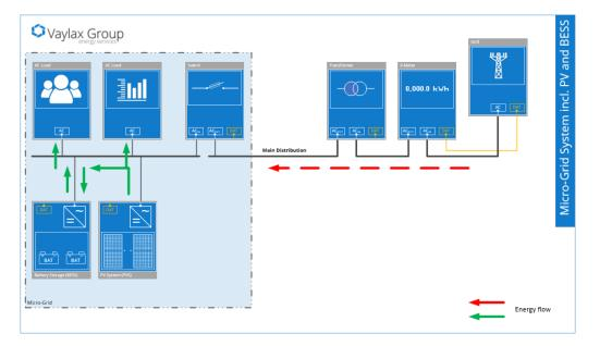
Designing a suitable Micro-grid requires a comprehensive grid and load study. The components suitable for a particular Micro-Grid may include other power sources like diesel gen-sets, wind turbines, biomass energy systems as well as waterpower systems – all depending on availability and suitability.
