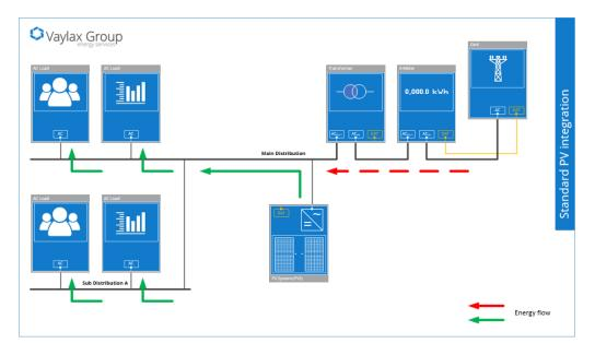
A grid-tied PV system attached to a consumer's infrastructure is technically designed in a way that its produced power will always be consumed first.
